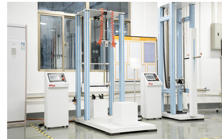
Frame vertical test
