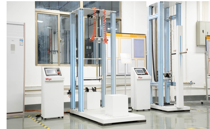
Frame vertical test
